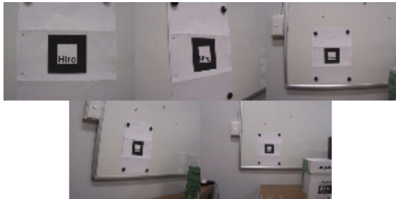
Figure 1: The ARToolkit marker used for registration for the Edge Detection Algorithm, in the five camera/marker positions, inside against a white interior wall
