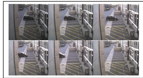
Figure 8 Illustration of increase in correlation coefficient when a vehicle pulls out of the parking space. From left to right: frame at 1sec, 4sec, 6sec, 8sec, 10sec, 15sec.
